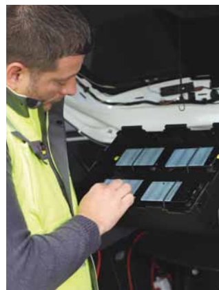
Each drivetest vehicle carried six Samsung Galaxy S9 smartphones.
