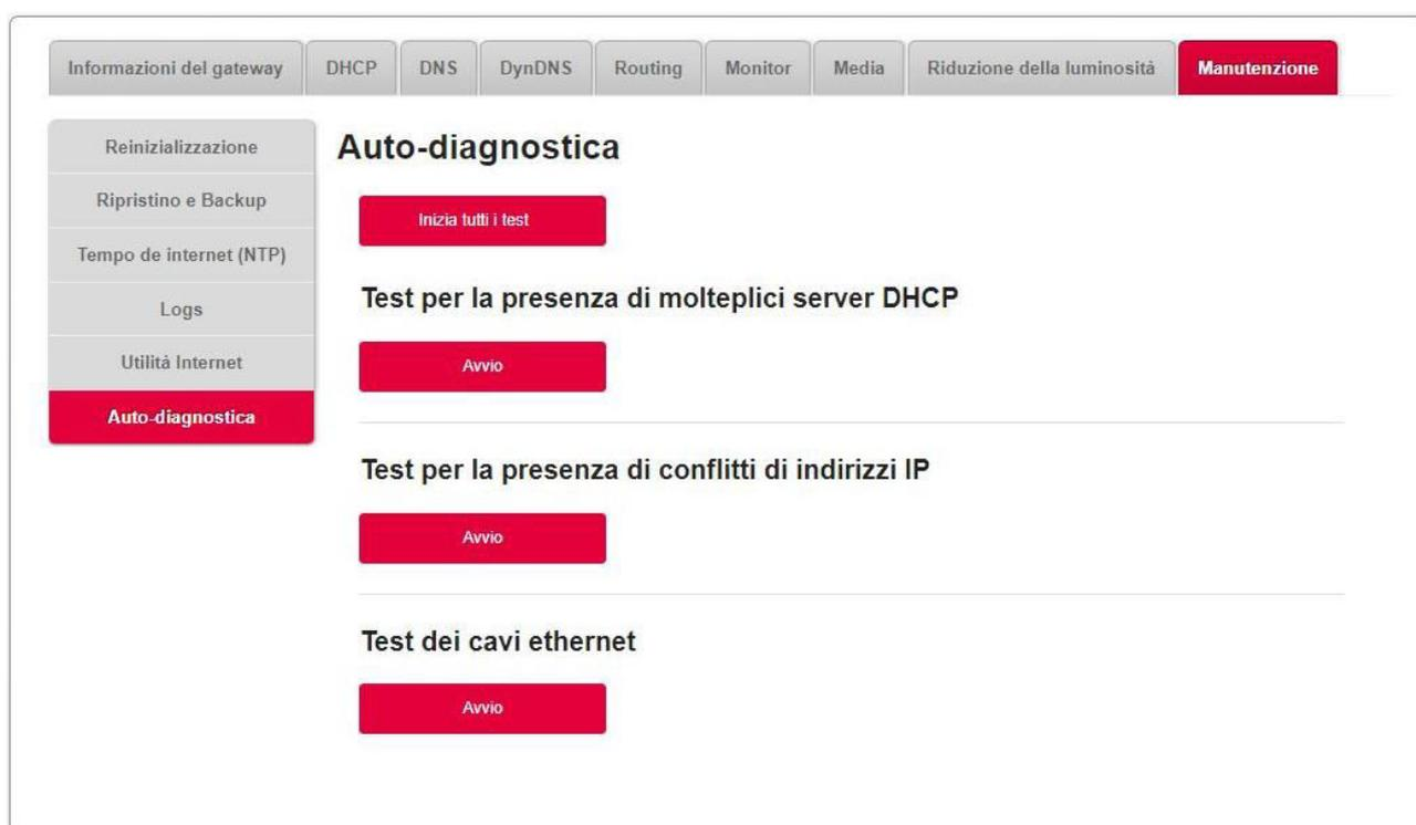
The screenshot shows the 'Auto-diagnostica' (Auto-Diagnostic) section of the Sunrise Internet Box interface. The 'Manutenzione' (Maintenance) tab is selected. Under the 'Auto-diagnostica' sub-tab, there are three test sections, each with a red 'Avvio' (Start) button:
