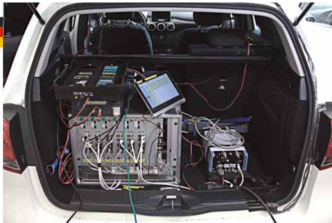
Both cars utilized for drive testing were equipped with eight Samsung Galaxy S5 each in order to assess voice service quality.
