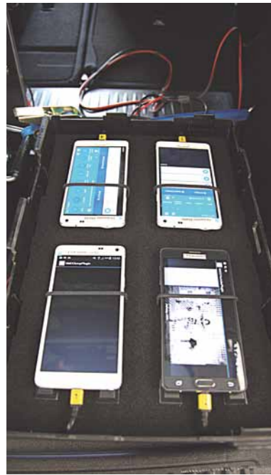
Four Samsung Galaxy Note 4 smartphones used to measure the data performance of cellular networks.
