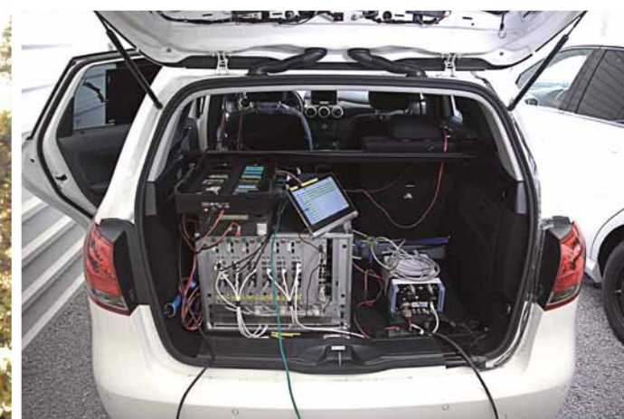
Each of the test vehicles carried up to twelve smartphones. They were controlled and monitored by the specialized test systems of P3.
