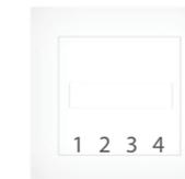
Remove the **protective caps** from both ends of the fibre cable and as well on the box. Open the cap on the fiber optic cable outlet (OTO socket). Plug one end of the cable into the communicated OTO-Slot (1-4) and the other end into the box.
